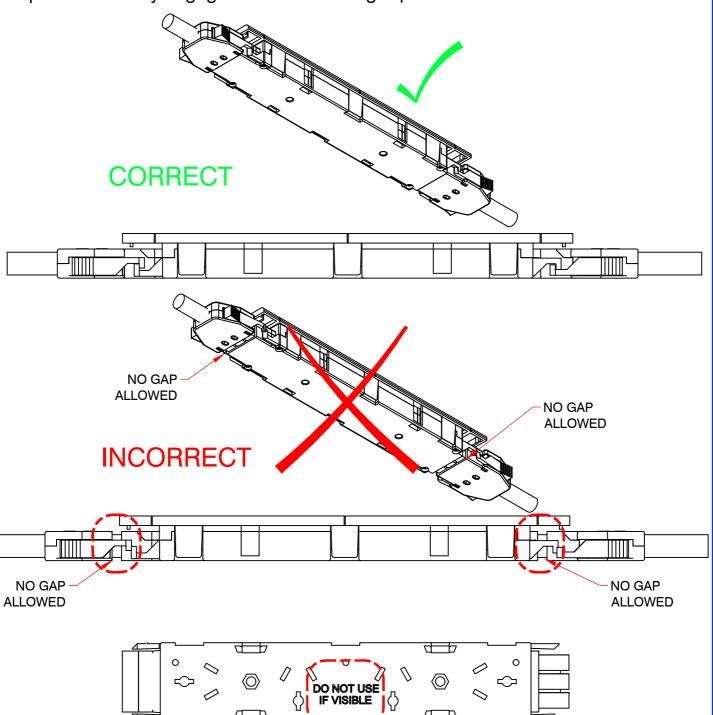
IF THE MARKING 'DO NOT USE IF VISIBLE' CAN BE SEEN, THE OUTLET DOES NOT HAVE THE FRONT FASCIA FIXED INTO POSITION AND THEREFORE MUST NOT BE USED. ATTACH THE FRONT FASCIA TO COMPLETE THE INSTALLATION
