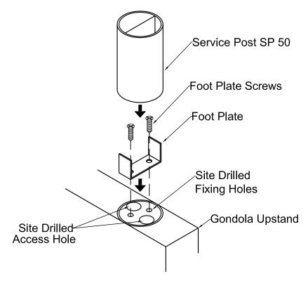
DETAIL OF SP 50 SERVICE POST FIXING TO COUNTER/GONDOLA
